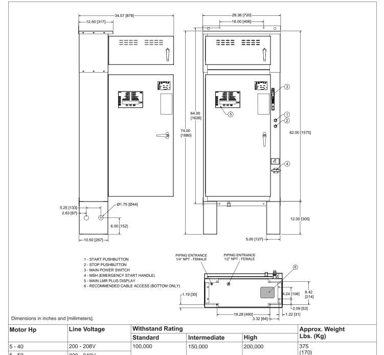
550 - 600V Coils Available: 380V-50Hz, 380V-60Hz, 415V-50Hz, 415V-60Hz
